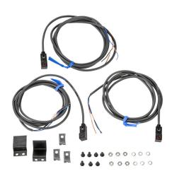
SureMotion inductive proximity sensor, rectangular, 8 x 7.4 x 17mm, polyarylate resin housing, top sensing, NPN, (2) N.C./(1) N.O. outputs, 2.5mm sensing distance, 1 kHz switching frequency, IP67, pigtail. Package of 3.
