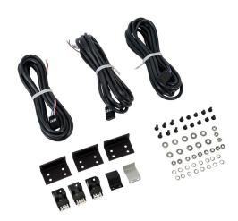
SureMotion photoelectric sensor, U-frame, PBT thermoplastic elastomer housing, through-beam, infrared light emission, 5mm sensing distance, 5-24 VDC operating voltage, selectable light-on/dark-on, PNP, 4-pole connector (direct solder).
