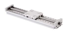
SureMotion linear actuator assembly, twin square bearing rail, 60mm wide, 210mm travel, ball screw, 10mm pitch, carbon steel rail.
