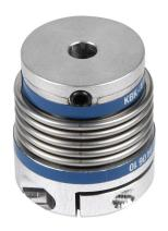
SureMotion drive coupling, bellows, aluminum alloy, clamp, size 20, 5 x 14mm bore. For use with LAHP-33 series actuators and SV2L-202 and SV2L-204 series servo motors.
