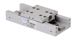
SureMotion linear slide assembly, single square bearing rail, 50mm wide, 52mm travel, carbon steel rail.
