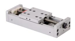
SureMotion linear actuator assembly, single square bearing rail, 50mm wide, 52mm travel, lead screw, 0.25in pitch, carbon steel rail.
