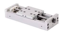
SureMotion linear actuator assembly, single square bearing rail, 50mm wide, 52mm travel, ball screw, 3mm pitch, carbon steel rail.
