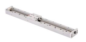
SureMotion linear actuator assembly, single square bearing rail, 50mm wide, 304mm travel, lead screw, 0.25in pitch, carbon steel rail.
