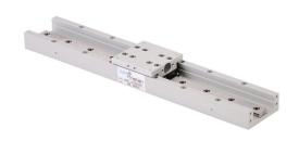
SureMotion linear slide assembly, single square bearing rail, 50mm wide, 220mm travel, carbon steel rail.
