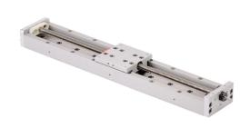
SureMotion linear actuator assembly, single square bearing rail, 50mm wide, 220mm travel, lead screw, 0.25in pitch, carbon steel rail.
