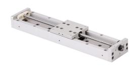
SureMotion linear actuator assembly, single square bearing rail, 50mm wide, 152mm travel, ball screw, 3mm pitch, carbon steel rail.
