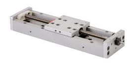
SureMotion linear actuator assembly, single square bearing rail, 50mm wide, 102mm travel, lead screw, 0.25in pitch, carbon steel rail.
