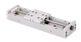
SureMotion linear actuator assembly, single square bearing rail, 50mm wide, 102mm travel, ball screw, 3mm pitch, carbon steel rail.
