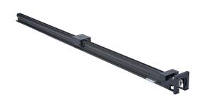
SureMotion linear actuator assembly, Gen 2 compact, 2.030in wide, 36in travel, lead screw, 1.0in pitch, hard coated aluminum rail.
