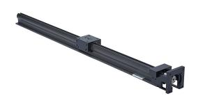
SureMotion linear actuator assembly, Gen 2 compact, 2.030in wide, 24in travel, lead screw, 0.5in pitch, hard coated aluminum rail.
