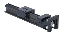
SureMotion linear actuator assembly, Gen 2 compact, 2.030in wide, 6in travel, lead screw, 0.5in pitch, hard coated aluminum rail.
