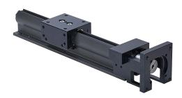
SureMotion linear actuator assembly, Gen 2 compact, 2.030in wide, 6in travel, lead screw, 1.0in pitch, hard coated aluminum rail.
