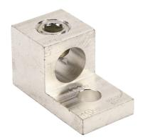
Penn-Union mechanical lug, box type, tin-plated aluminum, 600V, 1 openings, (1) 300-800 MCM copper or aluminum, AL9CU.
