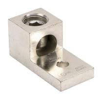
Penn-Union mechanical lug, box type, tin-plated aluminum, 600V, 1 openings, (1) 2 AWG-600 MCM stranded copper or aluminum, AL9CU.
