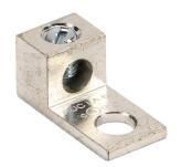
Penn-Union mechanical lug, box type, tin-plated aluminum, 600V, 1 openings, (1) 14-4 AWG stranded copper or (1) 8-4 AWG stranded aluminum, AL9CU.
