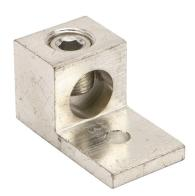
Penn-Union mechanical lug, box type, tin-plated aluminum, 600V, 1 openings, (1) 4 AWG-500 MCM stranded copper or aluminum, AL9CU.
