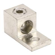
Penn-Union mechanical lug, box type, tin-plated aluminum, 600V, 1 openings, (1) 6 AWG stranded copper or aluminum-350 MCM copper or aluminum, AL9CU.
