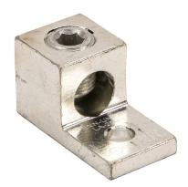
Penn-Union mechanical lug, box type, tin-plated aluminum, 600V, 1 openings, (1) 6 AWG stranded copper or aluminum-250 MCM copper or aluminum, AL9CU.
