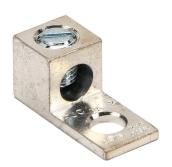
Penn-Union mechanical lug, box type, tin-plated aluminum, 600V, 1 openings, (1) 14-2 AWG stranded copper, (2) 14-10 AWG stranded copper, (1) 12-2 AWG stranded aluminum or (2) 10-12 AWG stranded aluminum, AL9CU.
