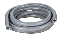
Electri-Flex Liquatite liquid-tight flexible metallic conduit, hot dipped galvanized steel, PVC jacket, 1in trade size, gray, UL-360 Listed, 25ft/7.6m coil length.
