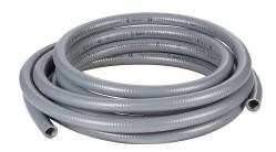
Electri-Flex Liquatite liquid-tight flexible metallic conduit, hot dipped galvanized steel, PVC jacket, 3/4in trade size, gray, UL-360 Listed, 25ft/7.6m coil length.
