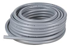
Electri-Flex Liquatite liquid-tight flexible metallic conduit, hot dipped galvanized steel, PVC jacket, 3/4in trade size, gray, UL-360 Listed, 100ft/30.4m coil length.
