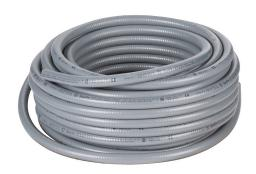
Electri-Flex Liquatite liquid-tight flexible metallic conduit, hot dipped galvanized steel, PVC jacket, 1/2in trade size, gray, UL-360 Listed, 100ft/30.4m coil length.
