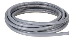
Electri-Flex Liquatite liquid-tight flexible metallic conduit, hot dipped galvanized steel, PVC jacket, 3/8in trade size, gray, UL-360 Listed, 25ft/7.6m coil length.
