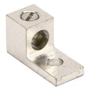
Penn-Union mechanical lug, box type, tin-plated aluminum, 600V, 1 openings, (1) 14-1/0 AWG stranded copper, (2) 14-4 AWG stranded copper, (1) 12-1/0 AWG stranded aluminum or (2) 12-4 AWG stranded aluminum, AL9CU.
