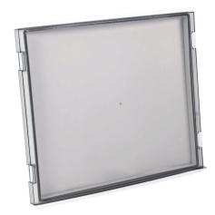
Fibox hinged enclosure window, 14.84 x 12.32in window, smoked polycarbonate, 14.84 x 12.32in frame, polycarbonate, RAL 7035 light gray, polyurethane gasket. For use with IP65 enclosures. Mounting hardware included.
