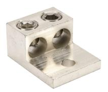
Penn-Union mechanical lug, box type, tin-plated aluminum, 600V, 2 openings, (1) 2 AWG stranded copper or aluminum-600 MCM copper or aluminum, AL9CU.
