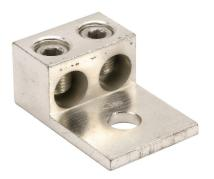
Penn-Union mechanical lug, box type, tin-plated aluminum, 600V, 2 openings, (1) 6 AWG stranded copper or aluminum-350 MCM copper or aluminum, AL9CU.
