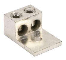
Penn-Union mechanical lug, box type, tin-plated aluminum, 600V, 2 openings, (1) 6 AWG stranded copper or aluminum-250 MCM copper or aluminum, AL9CU.
