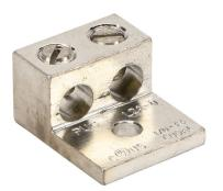
Penn-Union mechanical lug, box type, tin-plated aluminum, 600V, 2 openings, (1) 14-1/0 AWG stranded copper or (1) 8-1/0 AWG stranded aluminum, AL9CU.
