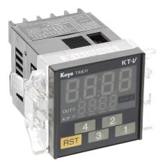
JTEKT multi-mode digital timer, two-line red/green LED display, fully selectable timing range, 10-30 VDC operating voltage, (1) NPN transistor and (1) SPDT relay output(s), 1/16 DIN mount, screw terminal(s). Panel mounting clip included.
