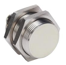
AutomationDirect inductive proximity sensor, tubular, 30mm diameter x 45mm body, 316 stainless steel housing, PNP, N.O. output, 15mm sensing distance, flush, 2 kHz switching frequency, IP65 IP66 IP67 IP68 IP69K, 4-pin M12 quick-disconnect.
