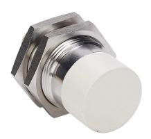
AutomationDirect inductive proximity sensor, tubular, 30mm diameter x 60mm body, 316 stainless steel housing, PNP, N.O. output, 30mm sensing distance, non-flush, 2 kHz switching frequency, IP65 IP66 IP67 IP68 IP69K, 4-pin M12 quick-disconnect.
