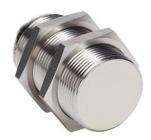
AutomationDirect inductive proximity sensor, tubular, 30mm diameter x 60mm body, 316 stainless steel housing, PNP, N.O. output, 15mm sensing distance, flush, 2 kHz switching frequency, IP65 IP66 IP67 IP68 IP69K, 4-pin M12 quick-disconnect.
