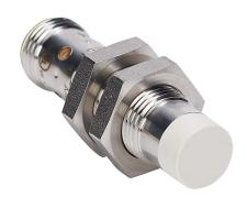
AutomationDirect inductive proximity sensor, tubular, 12mm diameter x 45mm body, 316 stainless steel housing, PNP, N.O. output, 10mm sensing distance, non-flush, 2 kHz switching frequency, IP65 IP66 IP67 IP68 IP69K, 4-pin M12 quick-disconnect.
