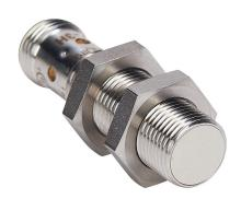
AutomationDirect inductive proximity sensor, tubular, 12mm diameter x 45mm body, 316 stainless steel housing, PNP, N.O. output, 4mm sensing distance, flush, 2 kHz switching frequency, IP65 IP66 IP67 IP68 IP69K, 4-pin M12 quick-disconnect.
