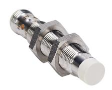
AutomationDirect inductive proximity sensor, tubular, 12mm diameter x 60mm body, 316 stainless steel housing, PNP, N.O. output, 10mm sensing distance, non-flush, 2 kHz switching frequency, IP65 IP66 IP67 IP68 IP69K, 4-pin M12 quick-disconnect.
