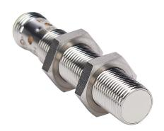
AutomationDirect inductive proximity sensor, tubular, 12mm diameter x 60mm body, 316 stainless steel housing, PNP, N.O. output, 4mm sensing distance, flush, 2 kHz switching frequency, IP65 IP66 IP67 IP68 IP69K, 4-pin M12 quick-disconnect.
