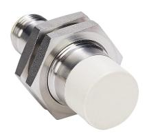
AutomationDirect inductive proximity sensor, tubular, 18mm diameter x 45mm body, 316 stainless steel housing, PNP, N.O. output, 12mm sensing distance, non-flush, 2 kHz switching frequency, IP65 IP66 IP67 IP68 IP69K, 4-pin M12 quick-disconnect.
