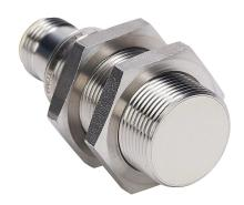
AutomationDirect inductive proximity sensor, tubular, 18mm diameter x 45mm body, 316 stainless steel housing, PNP, N.O. output, 8mm sensing distance, flush, 2 kHz switching frequency, IP65 IP66 IP67 IP68 IP69K, 4-pin M12 quick-disconnect.
