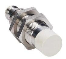
AutomationDirect inductive proximity sensor, tubular, 18mm diameter x 60mm body, 316 stainless steel housing, PNP, N.O. output, 15mm sensing distance, non-flush, 2 kHz switching frequency, IP65 IP66 IP67 IP68 IP69K, 4-pin M12 quick-disconnect.
