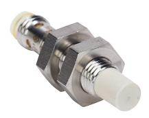
AutomationDirect inductive proximity sensor, tubular, 8mm diameter x 40mm body, 316 stainless steel housing, PNP, N.O. output, 6mm sensing distance, non-flush, 2 kHz switching frequency, IP65 IP66 IP67 IP68 IP69K, 3-pin M8 quick-disconnect.
