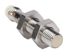
AutomationDirect inductive proximity sensor, tubular, 8mm diameter x 40mm body, 316 stainless steel housing, PNP, N.O. output, 3mm sensing distance, flush, 2 kHz switching frequency, IP65 IP66 IP67 IP68 IP69K, 3-pin M8 quick-disconnect.
