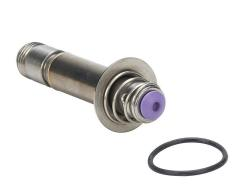
GC Valves rebuild kit, for use with NS301 series valves ending BE7, includes plunger-seat disc-spring assembly, plunger tube, operator O-ring and body O-ring.
