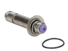
GC Valves rebuild kit, for use with NS301 series valves ending BE7, includes plunger-seat disc-spring assembly, plunger tube, operator O-ring and body O-ring.
