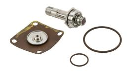
GC Valves rebuild kit, for use with S211 series AC valves ending V5EG5, includes diaphragm assembly, plunger assembly, plunger tube, plunger spring, body O-ring and operator O-ring.
